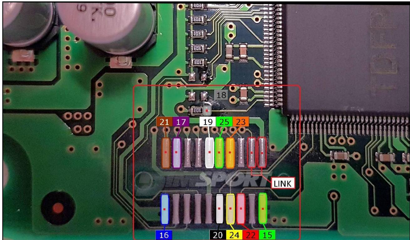
**F34NTA16 Soldering adapter connection      or**
